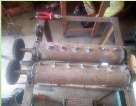
Figure 4. Fabricated and Sub-assembled of some components of the machine
