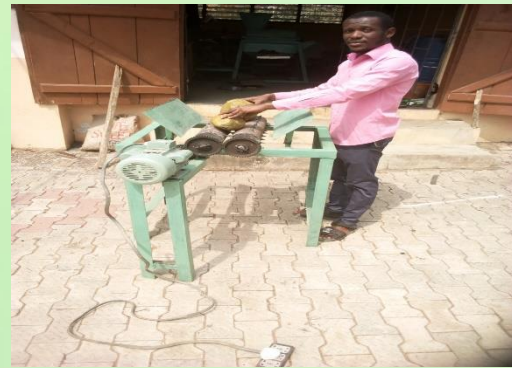
Figure 5. The dehusking machine under construction
