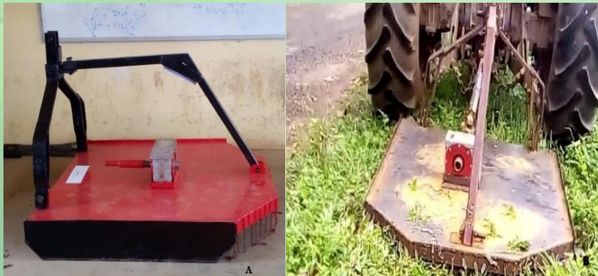
Figure 3. View of the fabricated Tractor-mounted rotary slasher (A) when completed (B) during operation before painting.
